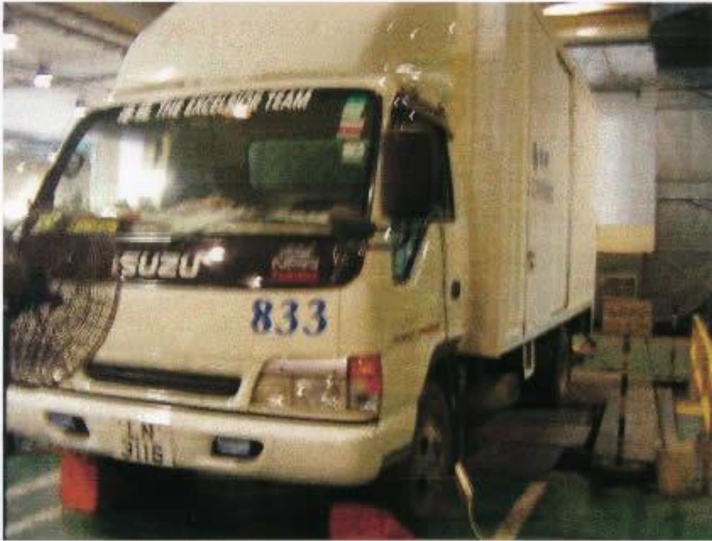
Photo 1 Testing vehicle in the chassis dynamometer with the external fuel tank (on the right).
